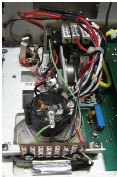
Figure 3: Power connections to the front panel
