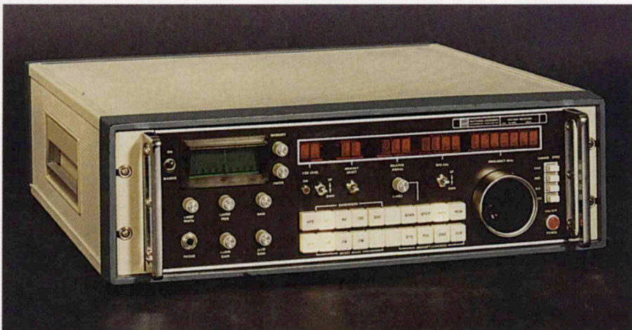
Watkins-Johnson's original WJ-8617 prototype. It was the world's first microprocessor-controlled, synthesized VHF/UHF radio. (Photo courtesy DRS Technologies)
