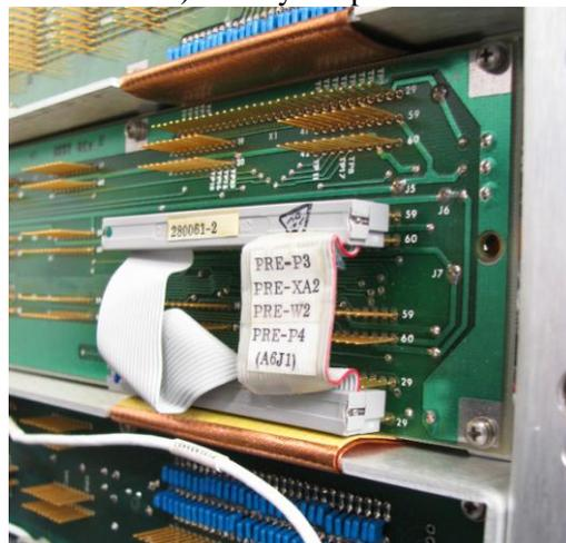
Figure 06: The PRE-W2 Cable assembly installed in the bottom of the A6 mainboard.
