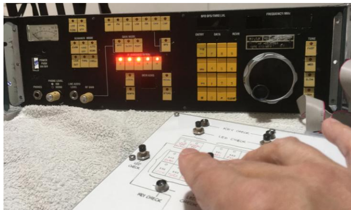
Figure 31: Bandwidth LEDs check.
