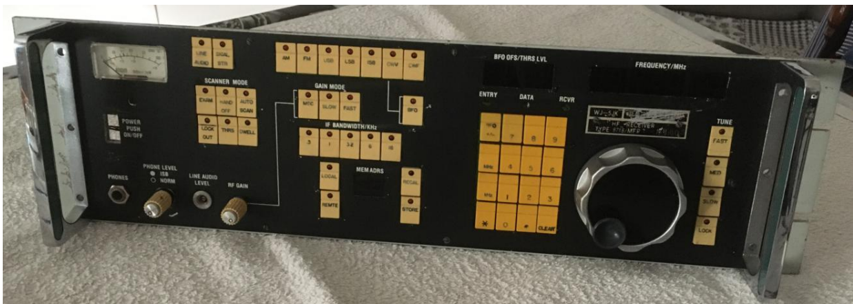
Figure 24: The partially restored Chinese MFP front panel. Please note that the two beige knobs in the left have been used temporarily only, the original ones are larger and black, look at Figure 1.
