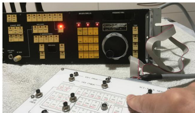
Figure 28: Service LEDs check.
