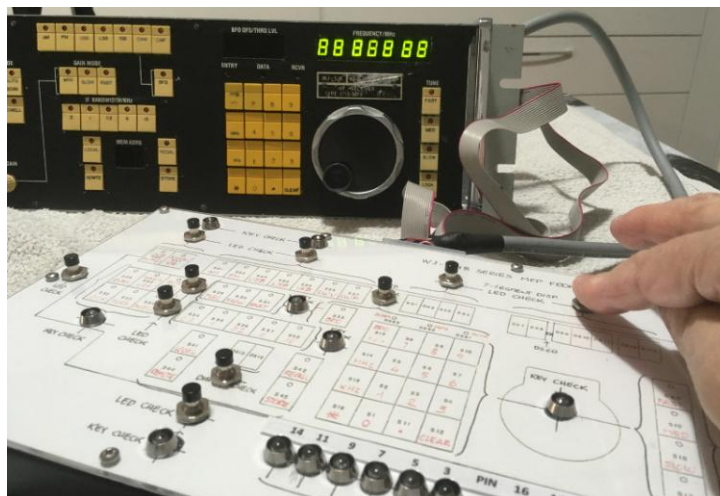
Figure 25: Frequency Display check.
