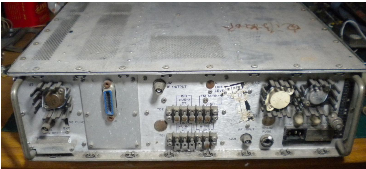
Figure 8: The rear panel of a WJ-5JK receiver is identical to the stock WJ-8718A/MFP one and seems to have been Factory built in the U.S.A.
