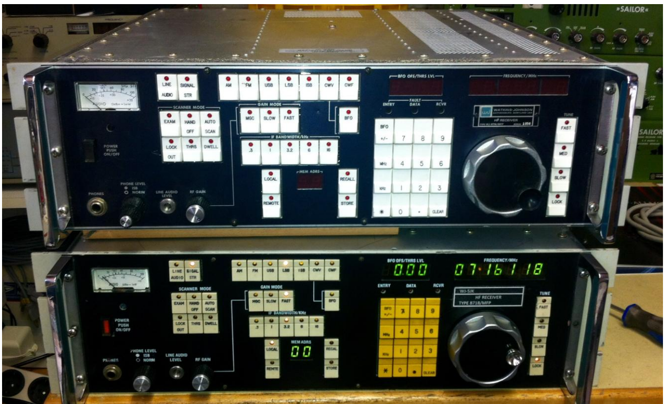
Figure 1: A stock WJ-8718A/MFP superimposed to its "Chinese" WJ-5JK version.
