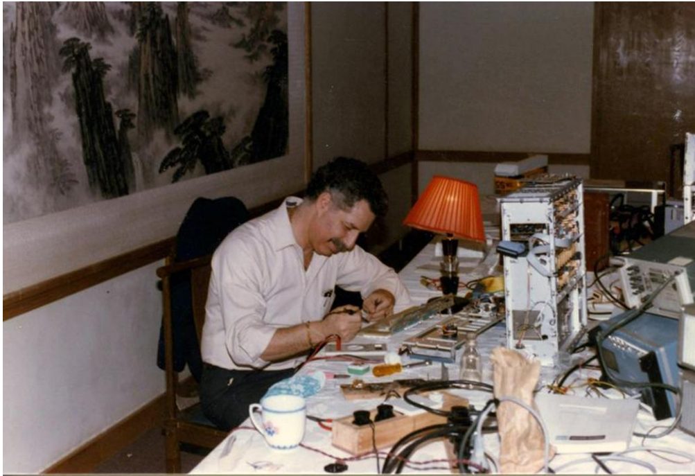
Figure 36: Mr. Bob Glaz is shown while repairing a front panel MFP PCB.
