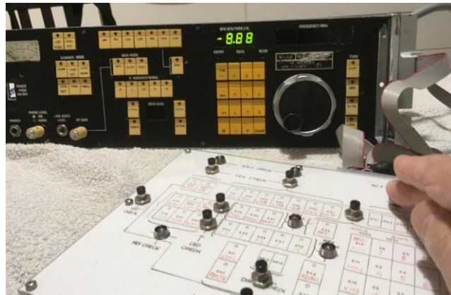
Figure 27: BFO Display check.
