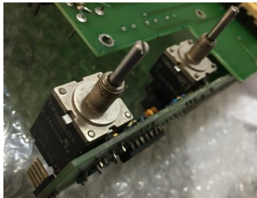
Figure 12: The Phone Level and the RF Gain control of the WJ-5JK have single knobs and miniature shafts.
