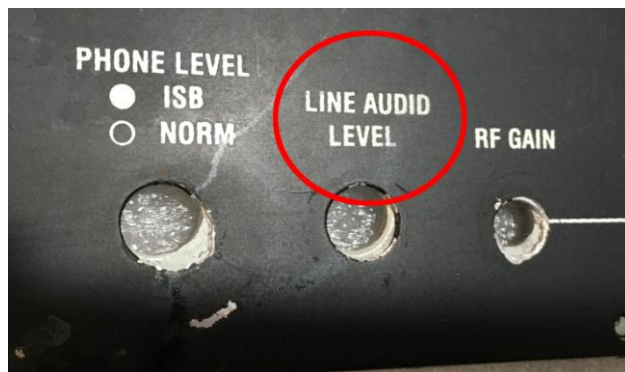
Figure 13: The “ AUDID ” misprint on the WJ-5JK front panel.
