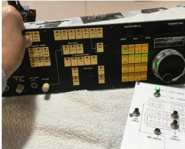
Figure 33: A successful switch check.
