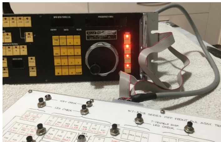
Figure 32: Tuning Rate LEDs check.
