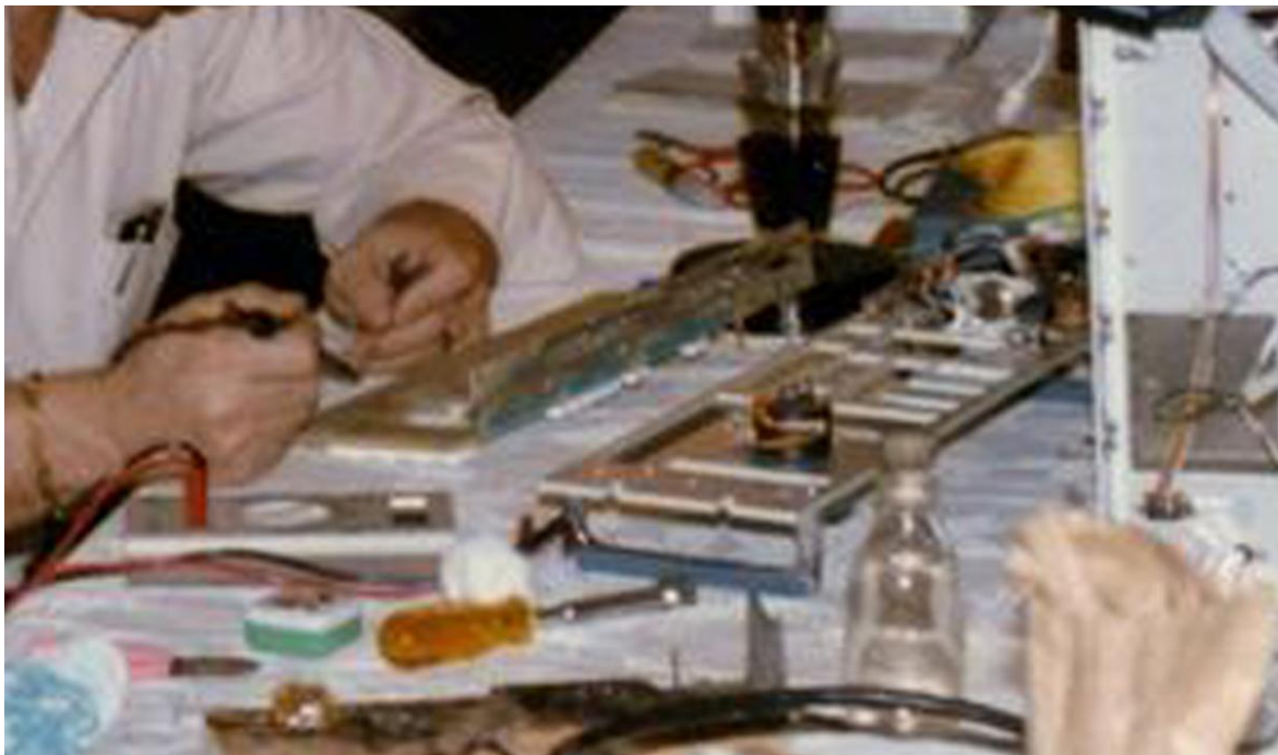
Figure 37: This picture enlargement shows clearly that Mr. Glaz is repairing an assembly formed by the Type 794309 MFP-A1A2 Front Panel Switch board and by the Type 794310 MFP-A1 Front Panel Switch/Encode board. Please notice that in both those boards there are no Tantalum capacitors!
