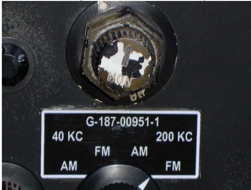
Fig. 4-29. Model G-187 Receiver, AGC "MON/DF" and Function Switches in the Front Panel.
