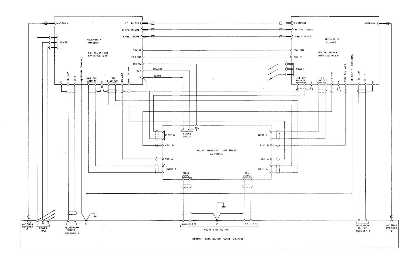
Typical Installation: ISB Space Diversity Receiving Terminal with FSK Facility
