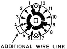
THIS IS A VIEW LOOKING FROM THE BACK OF THE AGC SWITCH. MODIFICATION APPLIES TO REAR WAFER ONLY.
