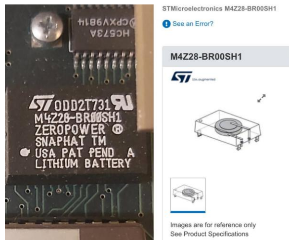
Figure 9: The battery IC of the Ten-Tec receivers (Data-Sheet at: https://www.mouser.it/datasheet/2/389/m4z28_br00sh-1849863.pdf ).
