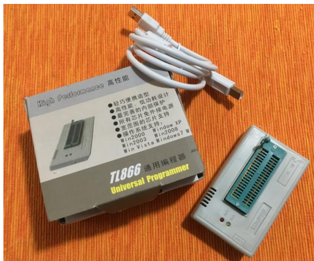
Figure 27: A cheap but very effective EPROM reader/copier/programmer that is easily found on the Internet. It can be used for programming NEW (or completely cancelled BLANK) EPROMs.
