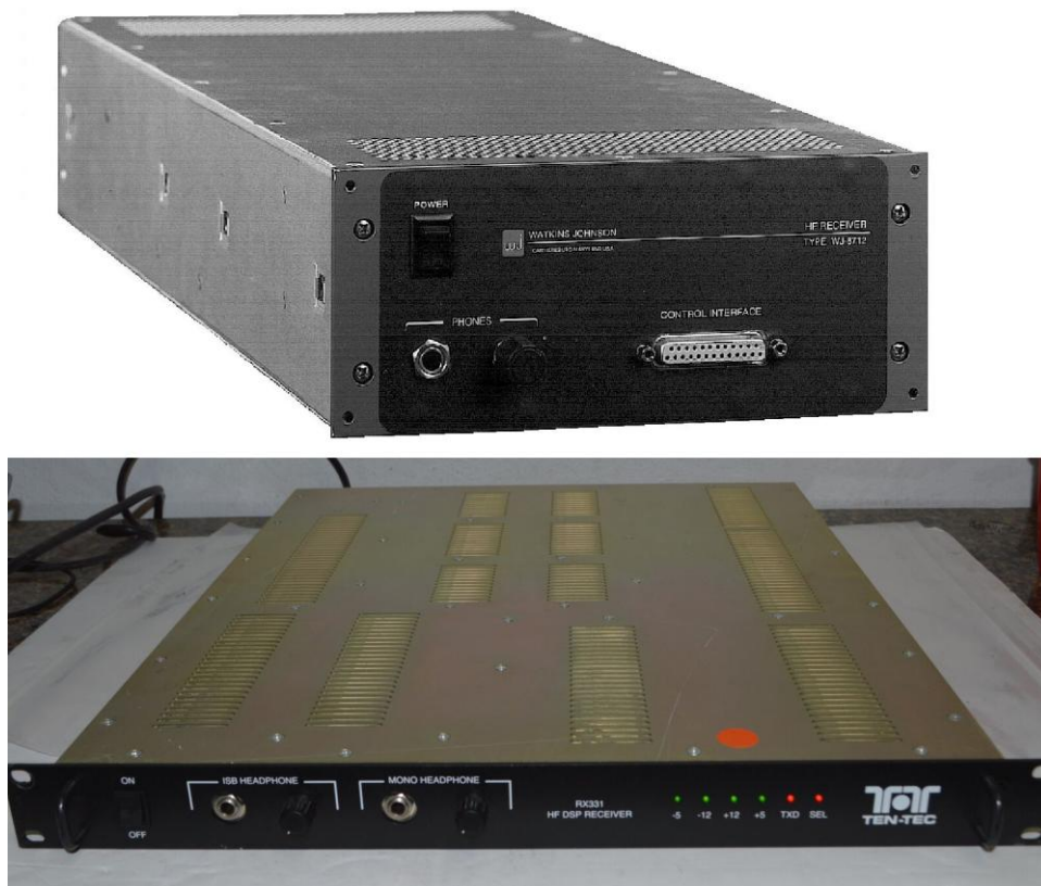
Figure 2: The WJ-8712A (above) and Ten-Tec RX-331 (below). While the Watkins-Johnson model is two rack units high and half wide, the Ten-Tec develops less in height (only one rack unit) and more in width (standard 19" rack). However, both receivers are quite deep (more than 20"-50 cm.).
