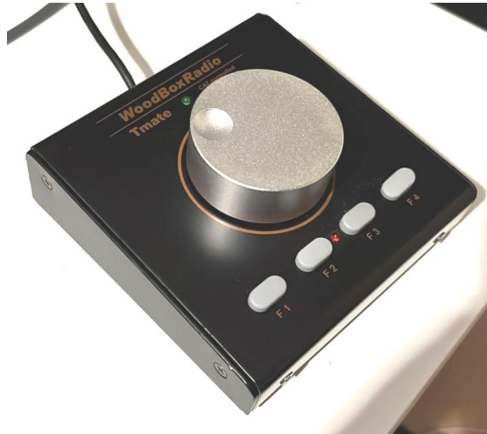
Figure 3: The Tmate unit of the WoodBoxRadio is shown here; it is one of the possible accessories which, together with a PC monitor, allow using the "black-box" receivers via an RS-232 interface.
