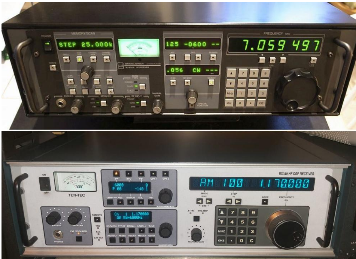
Figure 1: The WJ-8711A (above) and Ten-Tec RX-340 (below). Notice the similarity of the front panels of the two radios.
