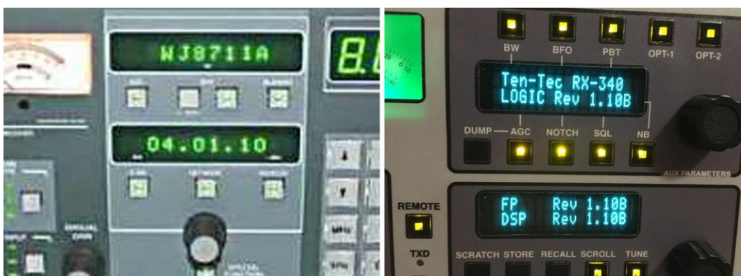
Figure 19: The "BITE" screens in the WJ-8711 (left) and in the Ten-Tec RX-340 (right).
