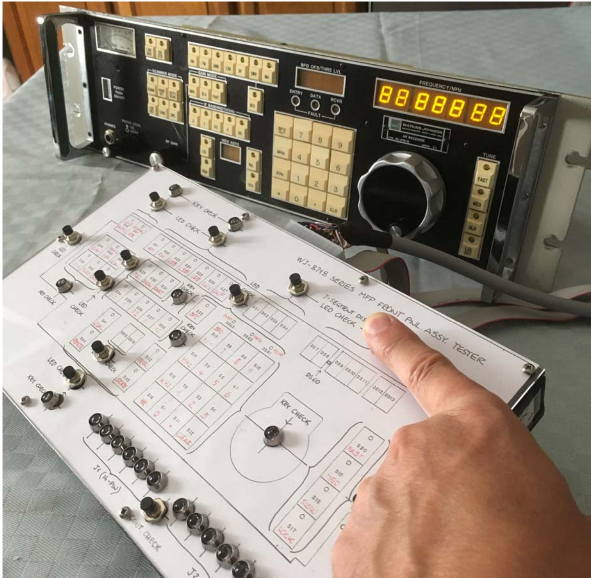
Figure 26: During a check of a WJ-8718-19FE front panel.
