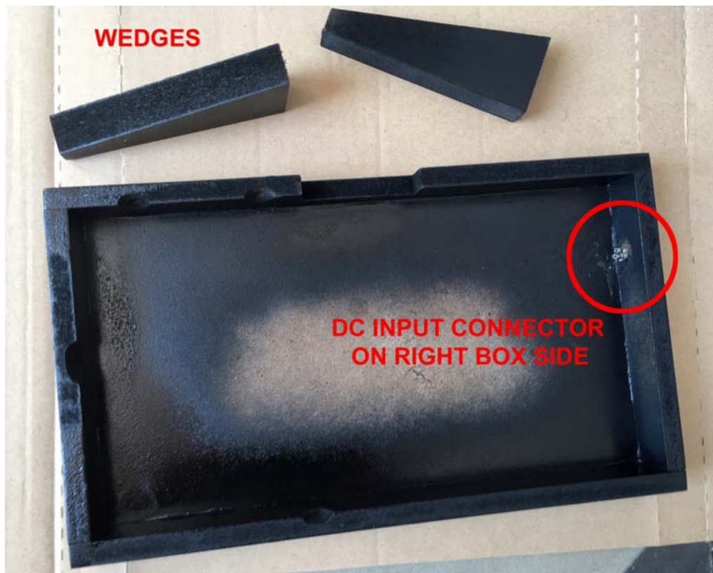
Figure 22: A picture of my black-painted wooden case for the MFP Tester Main Unit .
