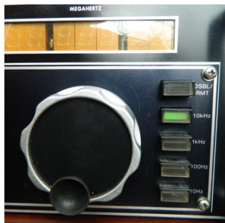
Figure 9: The “ DSBL/RMT ” ( Disable/Remote ) writing on a WJ-8718 MCM module.
