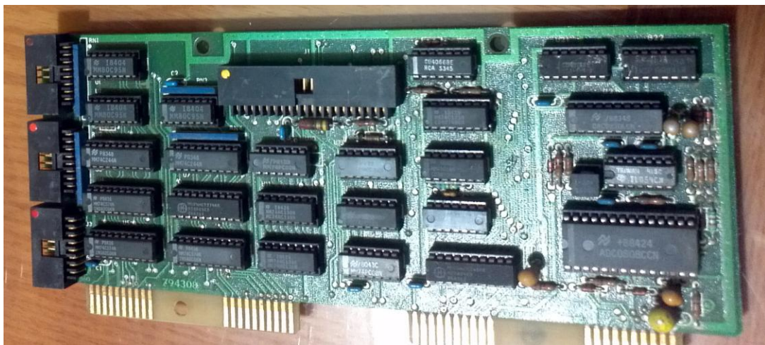
Figure 26: The later version (Type 794308-1) of the IF Interface card that has to be installed in the XA2 slots (X1 and X2).
