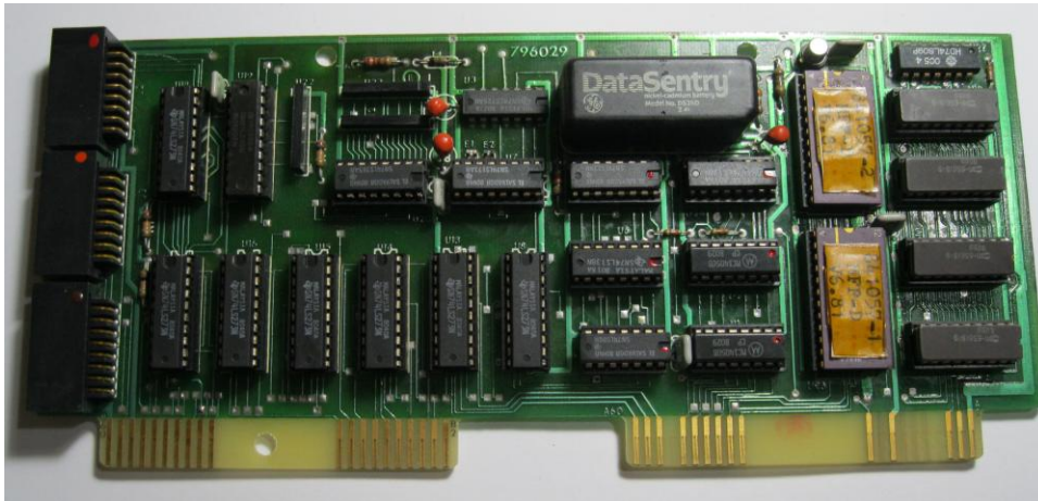
Figure 23: The Type 796029 Synthesizer Interface card that has to be installed in the XA1 slots (X7 and X8).
