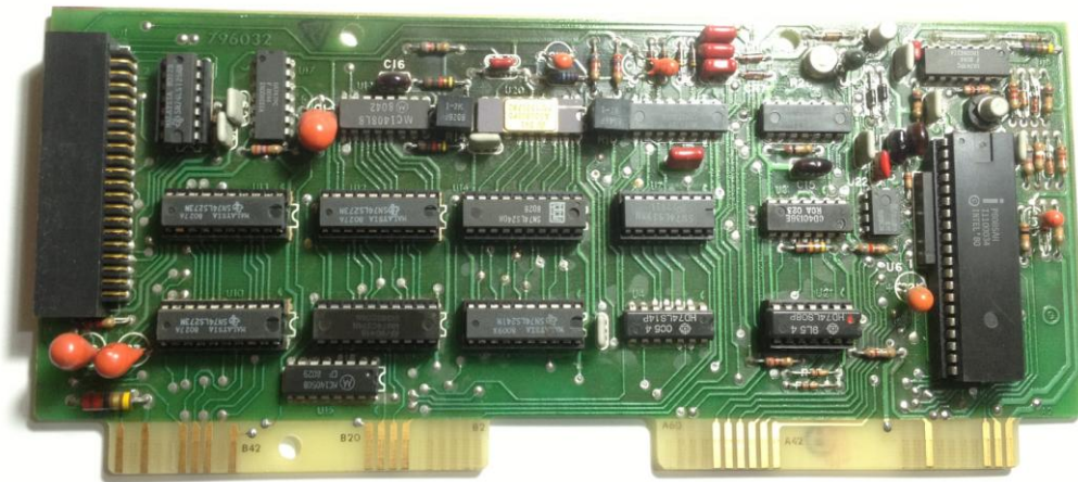
Figure 24: The Type 796032 IF Interface card that has to be installed in the XA2 slots (X1 and X2).
