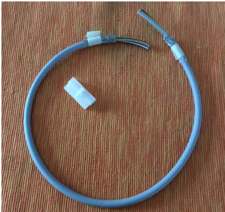
Figure 13: The 20-pole shielded cable cut at a length of about 65 cm.
